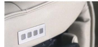
Integrated and concealed control panel placed on the right side of the seat cushion, when seated
